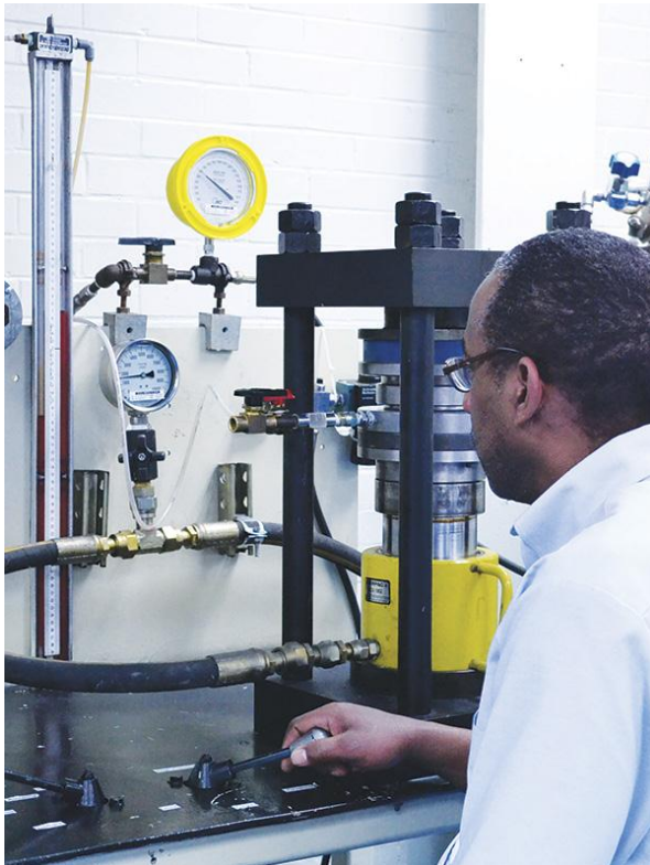
Image 1. A technician tests a gasket for leak tightness using DIN-3535 method and equipment. (Images and graphics courtesy of Garlock Sealing Technologies, LLC)
